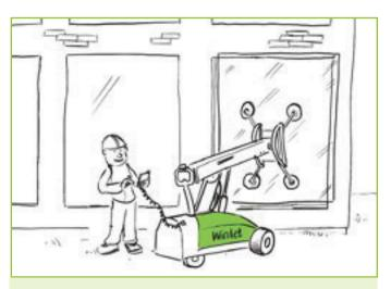
With a Winlet, glass installation is possible with just one operator.
